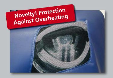
The **mesh fabric** in the Fiat front covers reliably prevents heat accumulation and possible damage to the headlamps.
